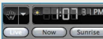
(**Sync** button: “**Live**” indicates an active connection, “**Off**” indicates there is no connection.)
